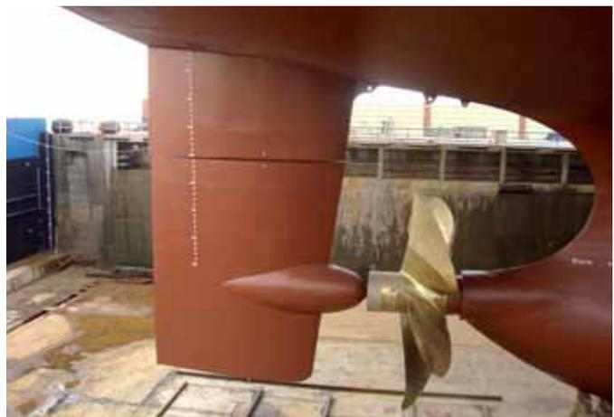
Five-bladed high screw propeller with Becker rudder
